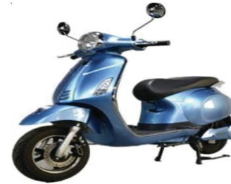
Model:JS000004 Brake: 48-60 front and rear disc brakes Controller: 12-tube 32A Motor: 10-inch 1000W motor
