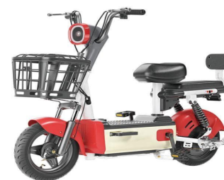
Model: TDT2311Z Motor: 350W Or 500W Controller: 48V 6-tube controller Tire: 14*2.5 Size: 1430*630*1030
