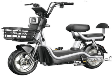
Model: TDT008Z Motor: 350W Or 500W Controller: 48V 6-tube controller Tire: 14*2.5 Size: 1485*685*958
