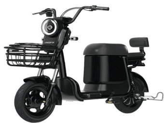
Model: TDT131Z Motor: 350W Or 500W Controller: 48V 6-tube controller Tire: 14*2.5 Size: 1459*590*1070
