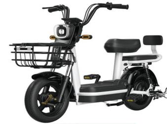
Model: TDT0006Z Motor: 350W Or 500W Controller: 48V 6-tube controller Tire: 14*2.5 Size: 1460*640*1055
