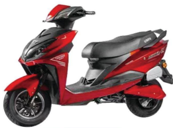
Model:JS000014 Brake: 60-72 front and rear disc brakes Controller: 15-tube 38A Motor: 10-inch 1500W motor
